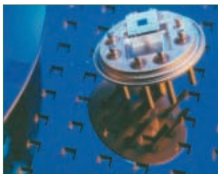
Figure 3. Manifold absolute pressure sensor uses anodic bonding (Robert Bosch GmbH)
