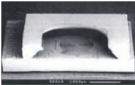
Figure 1. SEM shows cutaway of a packaged automotive gyroscope using glass frit bonding (Robert Bosch GmbH)
